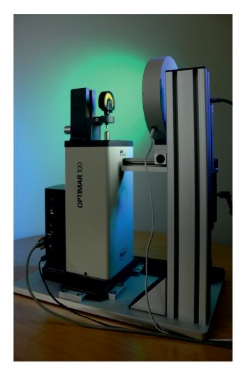
**QMSOFT**® supports not only conventional but also state-of-the-art calibration technologies such as optical and mechanical scanning methods (for example for calibrating cylindrical or tapered thread gauges) or image processing for the automated calibration of analogue and digital dial gauges.
